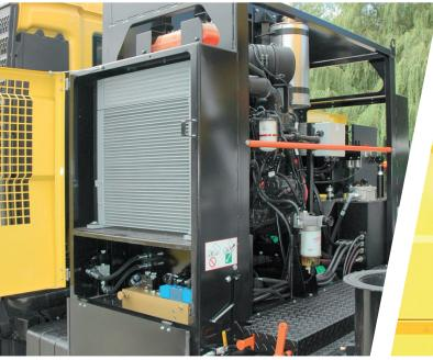
Easy access to auxiliary engine and all filters and fluid filler / top-up points.
