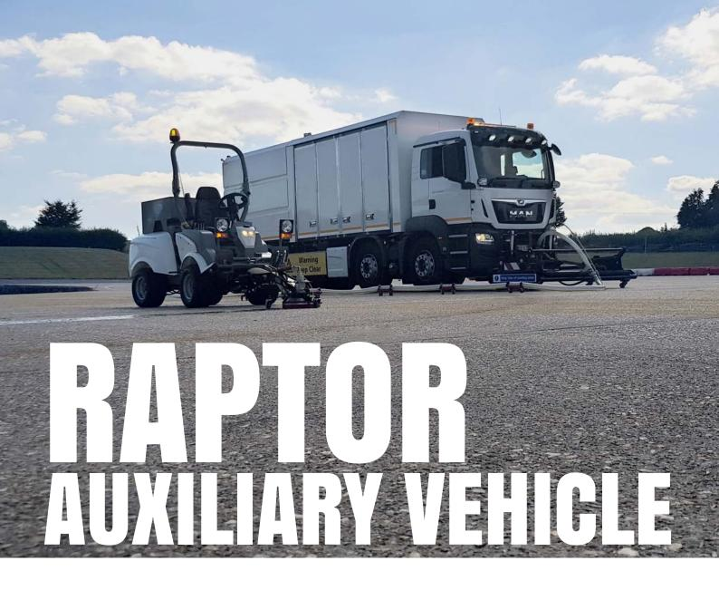
The Raptor is designed as a remote operating tool, increasing the versatility of the Jetting Systems Osprey. The Raptor may be fitted with articulating single arm for line marking removal or with a rubber removal / large surface area cleaning unit for surface cleaning in tight areas.
