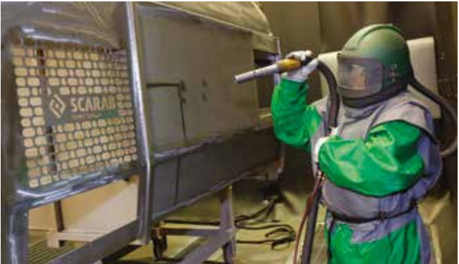
Shot blasting the stainless steel hopper
