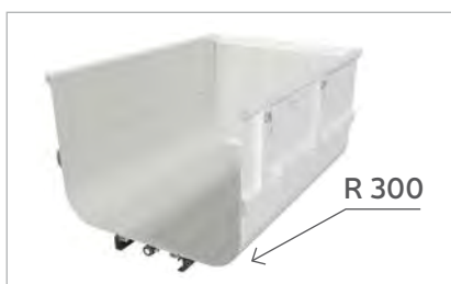
Container bottom to sides jointed with rounded shape metal sheet to avoid accumulation of dirt or waterlogging.
