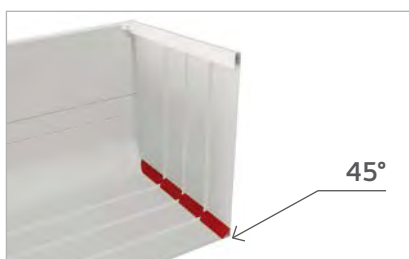
Container bottom to head metal sheet, jointed with 45° angle to avoid accumulation of dirt or waterlogging.
